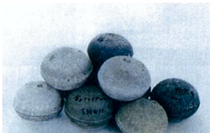
Solidification of incinerated ashes and burned ashes.
